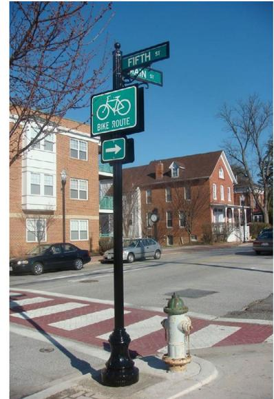
*When multiple signs are required, they should be clustered onto one pole when feasible.*
